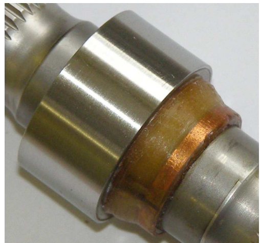
Fig. 2. Assembled torque transducer
